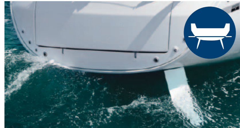
Double rudder blades ensure true to course steering, even under difficult conditions.
