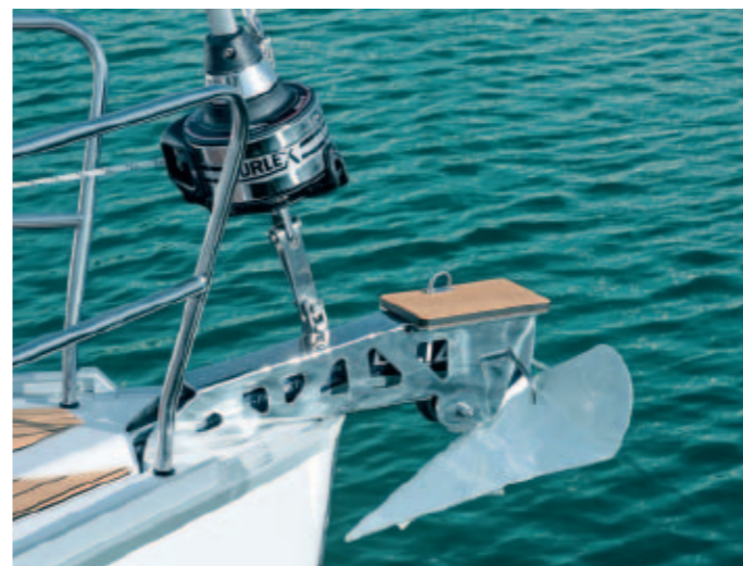
The gennaker bow roller is safe to reach from the foredeck.
